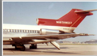
Iconic Rear Stair access/ egress on early B727s
